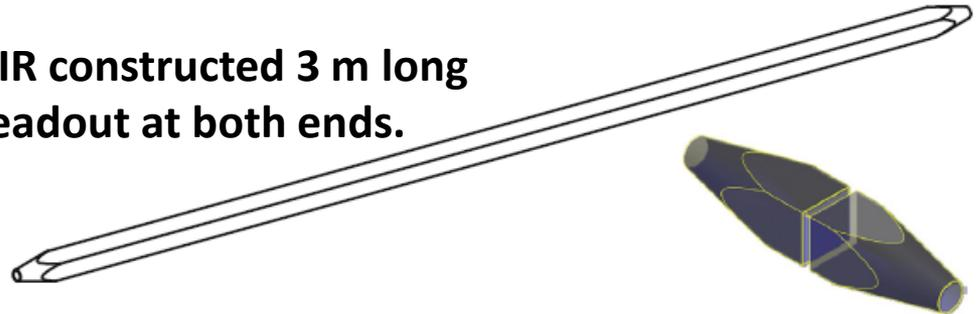
Fig. 1. NeuLAND bar. The left side shows the entire, 270 cm long NeuLAND bar. The right side shows the two tapered sides converting from  $5 \times 5 \text{ cm}^2$  square shape to  $d=2.5 \text{ cm}$  circular shape.
