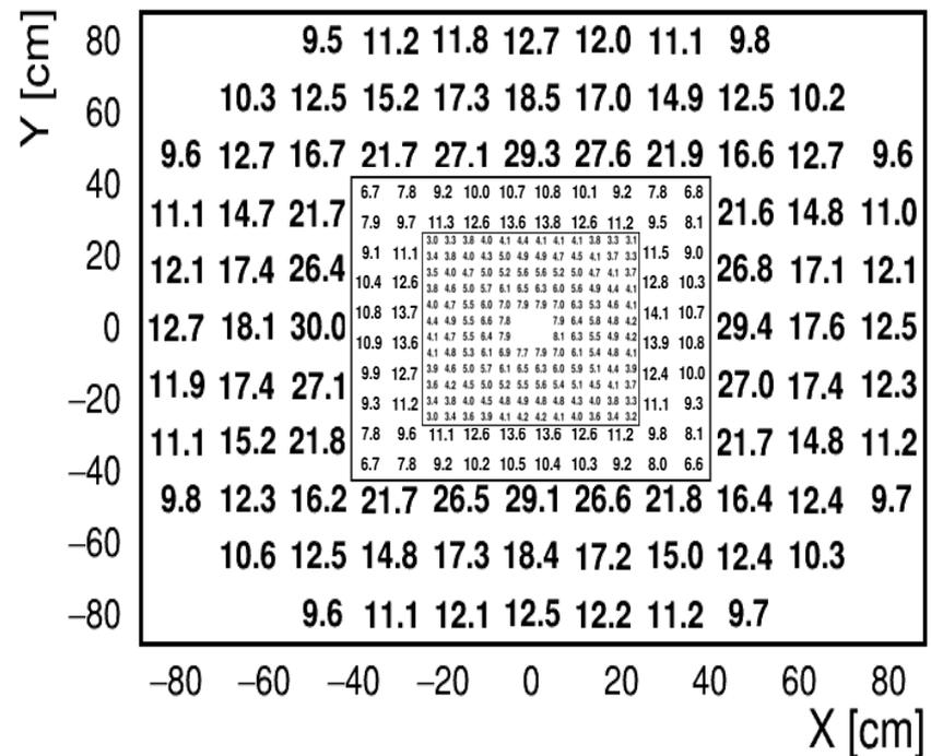
Result of simulation in HGEANT framework. Occupancy for Ag-beam is a factor  $\sim 1.7$  lower than for Au-beam, but achieves 30% in large cells.
