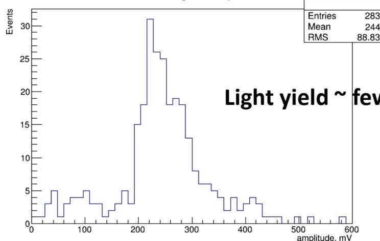
XP2262 signal amplitude (attenuation 10dB)
