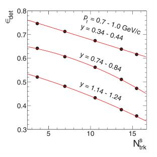
FIG. 11. Simulated proton detection efficiency  $\epsilon_{det}$  as a function of the number of reconstructed tracks per sector  $N_{trk}^s$ , shown here for three out of the 40 narrow phase-space bins used in our analysis. Efficiency points correspond to 2-fm-wide impact-parameter slices centered at b = 9, 7, 5, 3, and 1 fm, respectively; curves are the polynomials adjusted to model the occupancy dependence of the efficiency.
