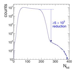
FIG. 2. Distribution of the total number of hits in the HADES time-of-flight detectors TOF and RPC in the 43% most central Au + Au events accepted by the PT3 trigger. The tiny contribution of order  $\leq 2 \times 10^{-4}$ , visible for  $N_{\text{hit}} > 260$ , is attributed to event pileup.
