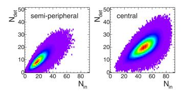
FIG. 12. Proton response matrices of the HADES detector simulated with IQMD clustering for two centrality selections, semiperipheral (30–40%) and central (0–10%). These matrices encode the distribution of the number  $N_{det}$  of reconstructed proton tracks within the phase-space bin of interest (here  $y \in y_0 \pm 0.5$ )—for any given number  $N_{in}$  of protons emitted into this bin.
