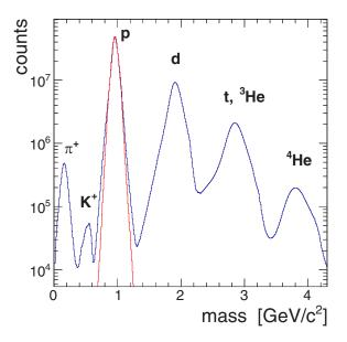
FIG. 7. Particle mass distribution of reconstructed tracks—as deduced from particle velocity, momentum, and energy loss—for positive particles within the phase-space bin of interest ( $y = y_0 \pm 0.5$  and  $0.4 < p_t < 1.6 \text{ GeV}/c$ ). The masses selected by the proton cut (see Fig. 6) as well as the Z = 1 condition are shown in red. Contaminations from lower masses ( $\pi^+$ , K<sup>+</sup>) and higher masses (d, t, He) are below 0.1%, resulting in an overall proton purity >0.999.
