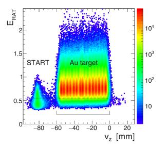
FIG. 4. Ratio of transverse to longitudinal energy  $E_{RAT}$  as a function of the reconstructed event vertex along the beam axis *z*. The horizontal dashed line indicates the  $E_{RAT} > 0.55$  cut used to further suppress Au + C reactions in the Kapton strips of the target holder. The solid line delimits the vertex cut applied on the target region.
