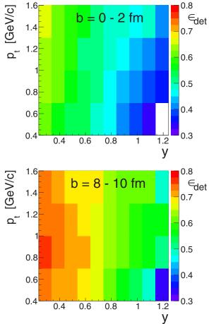
FIG. 10. Simulated proton detection efficiency  $\epsilon_{det}$  in one sector of HADES as a function of rapidity y and transverse momentum  $p_t$ , and for two impact parameter ranges (left, b = 8-10 fm and right, b = 0-2 fm).
