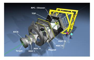
FIG. 1. Schematic explosion view of the HADES experiment. The forward wall hodoscope (FWALL) used for centrality selection (see text) is not shown on this picture.
