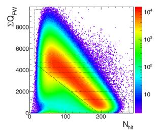
FIG. 5. Sum signal  $\Sigma Q_{FW}$  measured in the forward wall vs number of hits  $N_{hit}$  in the TOF and RPC. The black long-dashed line indicates a loose 2D cleaning cut applied to remove the contamination from peripheral events. Centrality selections, e.g., in steps of 5%, were done by applying additional, more restrictive cuts on  $\Sigma Q_{FW}$  as indicated by the set of short-dashed horizontal lines.
