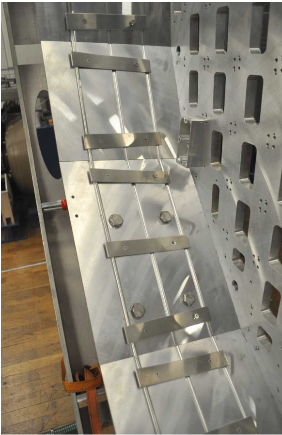
Figure 5.37: Cut outs in the stiffener ring of the forward endcap to accommodate the cooling lines of the side cooling. Left milling with inserted aluminum tube. In the middle and on the right the cut outs are without tubes [4].
