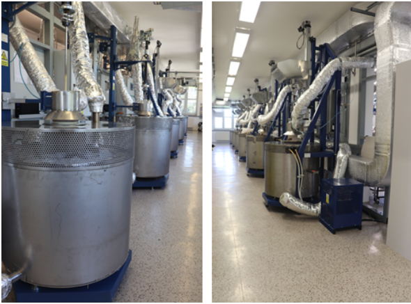
Figure 2.8: Photograph of the installed furnaces at CRYTUR for PWO-II crystal growing.
