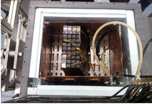
Figure 7.2: Front view of a partly mounted PROTO120 without front thermal insulation panel. The crystals are surrounded by cooling plates and thermal insulation.
