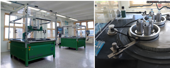
Figure 2.9: Photograph of the equipment installed at CRYTUR for polishing PWO-II crystals.
